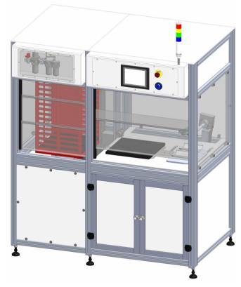
The system is totally closed in a protected environment for safety and equipped with ionized air control to avoid electric charges formation.
