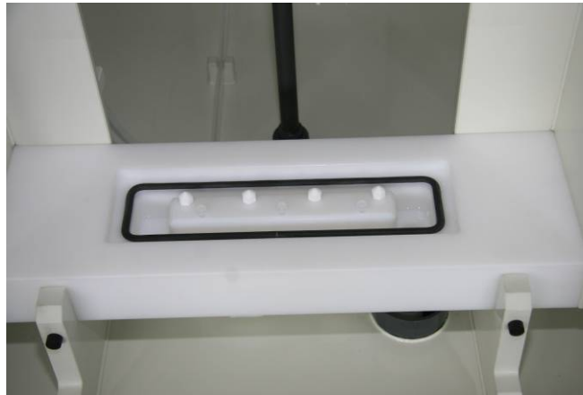
Bottom flange with PTFE nozzles
