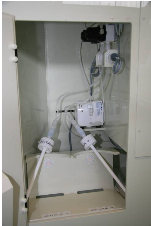
Filling system from bottle (model without CDS filling)
