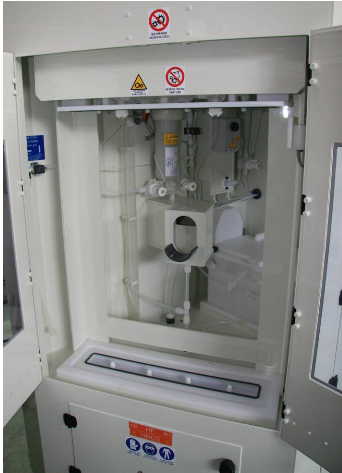
Top automatic sealing flange with PTFE special atomizing nozzles
