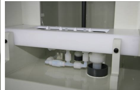
Exhaust extracion - Chamber presence sensor
