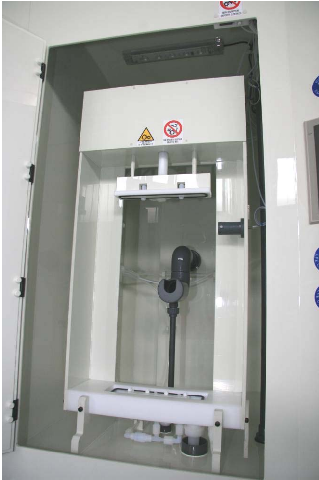
Top automatic sealing flange with PTFE special atomizing nozzles
