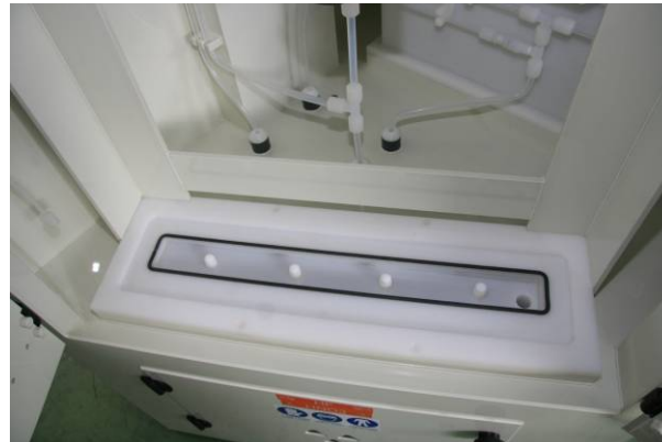
Bottom flange with PTFE nozzles
