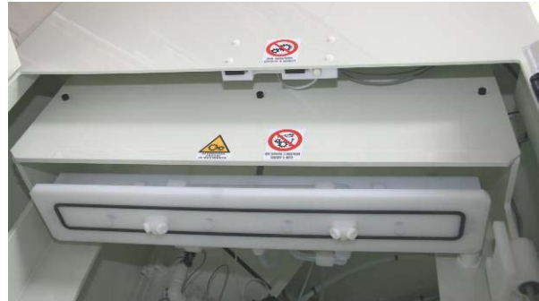
Top automatic sealing flange with PTFE special atomizing nozzles
