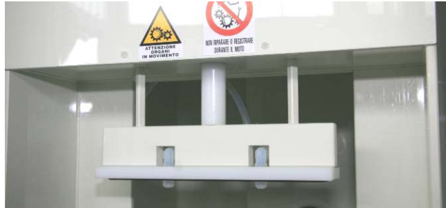
Top automatic sealing flange with PTFE special atomizing nozzles
