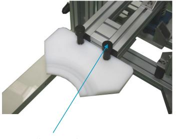
Plastic fasteners for support locking (no tools needed for support change operations)
