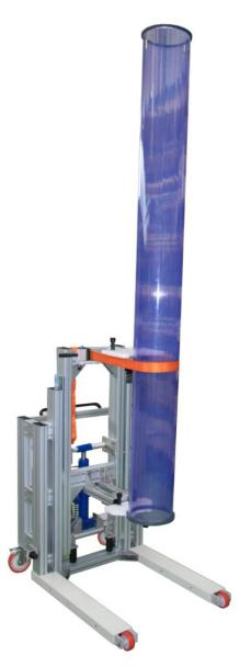
This trolley has been designed with the purpose of quartz tubes insertion into the cleaning equipment.
