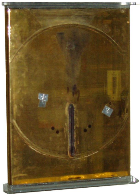
LPE 3061 chamber and Process kit for EPI with special parts holder
