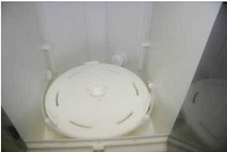
Rotary plateau to clean belljar saving chemicals
