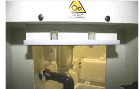
Automatic enclosyng system to clean ASM chambers only inside
