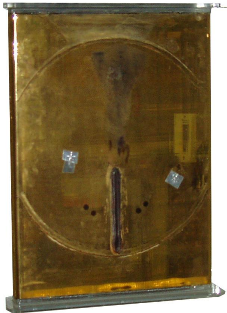
LPE 3061 chamber, LPE 2061 Quartz belljar and Process kit for EPI with special parts holder
