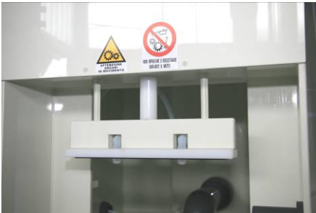
Automatic sealing cover for inside only chambers cleaning
