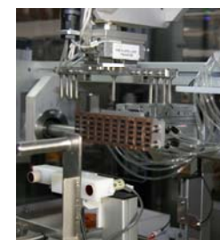
9. Y AXIS MOVES UP TO THE MANIFOLD
