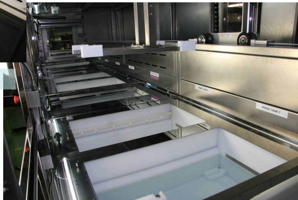
Overflow with level sensor
