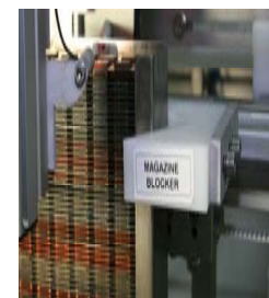
4. OPTICAL FIBER DETECTS LEADFRAME PRESENCE
