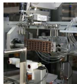
8. Y AXIS MOVES UP TO THE MANIFOLD
