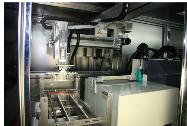
3. Z AXIS GOES UP AND X AXIS MOVE ON THE RIGHT (UP TO WJ CONVEYOR).
