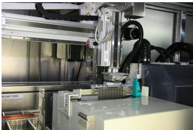
4. Z AXIS GOES DOWN ON THE CONVEYOR ENTRANCE. WAIT FOR CHAIN PIN.
