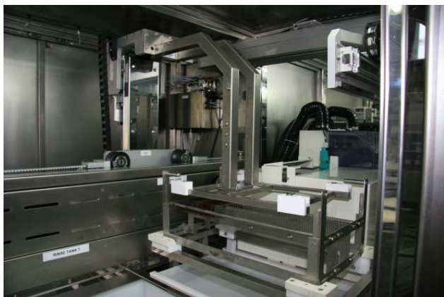
1. TANKS ROBOT DEPOSE THE CARRIER ON THE BUFFER STATION. Waterjet conveyor guides and chain will change dimension/steps according with leadframe format.
