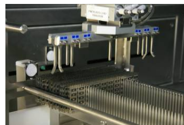
13. GRIPPER RELEASE THE LEADFRAME AND Z AXIS GOES UP FOR NEXT CATCHING
