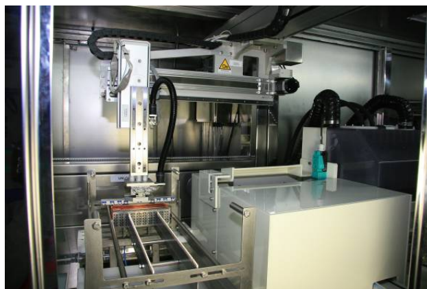
2. X AXIS MOVE ON THE LEFT AND Z AXIS GOES DOWN TO THE FIRST LEADFRAME. A PNE GRIPPER CATCHES THE LEADFRAME.
