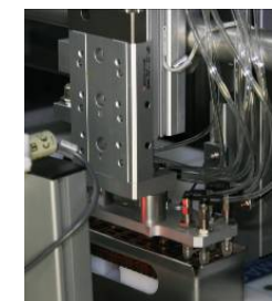
5. MANIFOLD MOVES DOWN TO CATCH LEADFRAMES. Vacuum presence check
