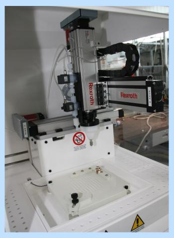
The System is composed by a Cartesian robot with three interpolated axes; it is extremely flexible and ensures high precision and repeatability of the operations.
